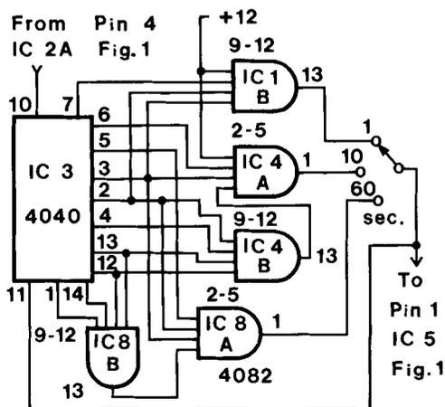
FIG. 2. Schematic circuit of the 50-Hz AC divider section to be inserted in Fig. 1 (for use in Europe) instead of the corresponding American (60-Hz) circuit consisting of IC 3, IC 1B, and IC 4A and B. The same power connections are used as in Fig. 1; in addition IC 8 requires +12V at pin 14 and ground at pin 7.
