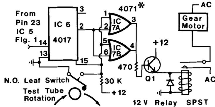
FIG. 3. Schematic circuit of the test-tube position sensor and motor turn-on interval control section of the fraction collector that will accommodate various gear motors of  $<2$  rpm. \*Pins 7, 12 and 13 of IC 7 and pin 8 of IC 6 are connected to ground while pin 16 of IC 6 and pin 14 of IC 7 are connected to +12 V (DC).
