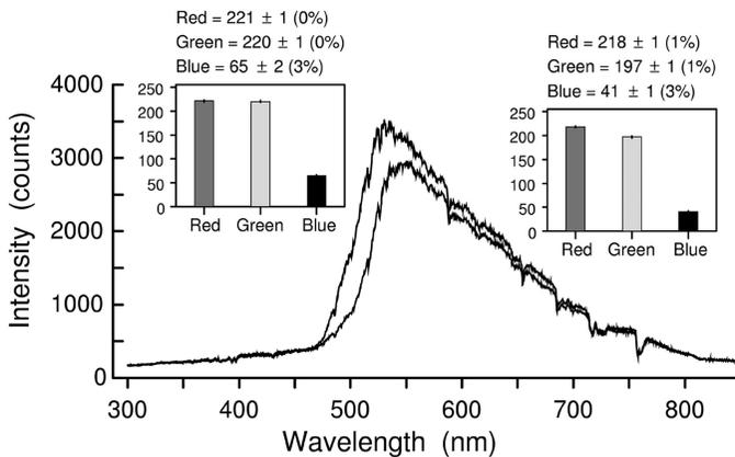
**Fig. 6.** Overlaid spectrograms (USB2000 spectroradiometer) of sunlight reflected from each of two yellow plastic sheets used in insect traps. The left inset of RGB values corresponds to the first sheet A with its spectrum shown offset to the left and higher, whereas the second sheet B corresponds to the inset on the right with a spectrum shifted to the right and slightly lower (RGB analysis of images taken by Nikon 2100, 18 February 2005 at 1130 hours, yellow sheets as in Table 2).
