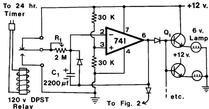
FIG. 1. Light intensity control for DC lamps. List of components—Resistors,  $\frac{1}{4}$  watt: (2) 30 K $\Omega$ ; Potentiometers: (1) 2 M $\Omega$ ; Capacitor: (1) 2200  $\mu$ f electrolytic 16 V; Transistors: (one per lamp) npn 2N3055 heat-sinked; Diodes: (3) IN4001; Integrated Circuit: (1) LM741; Lamps: 6 volt, 6 candlepower; Timer: (1) standard 24-h; Relay: (1) DPST 120 V.
