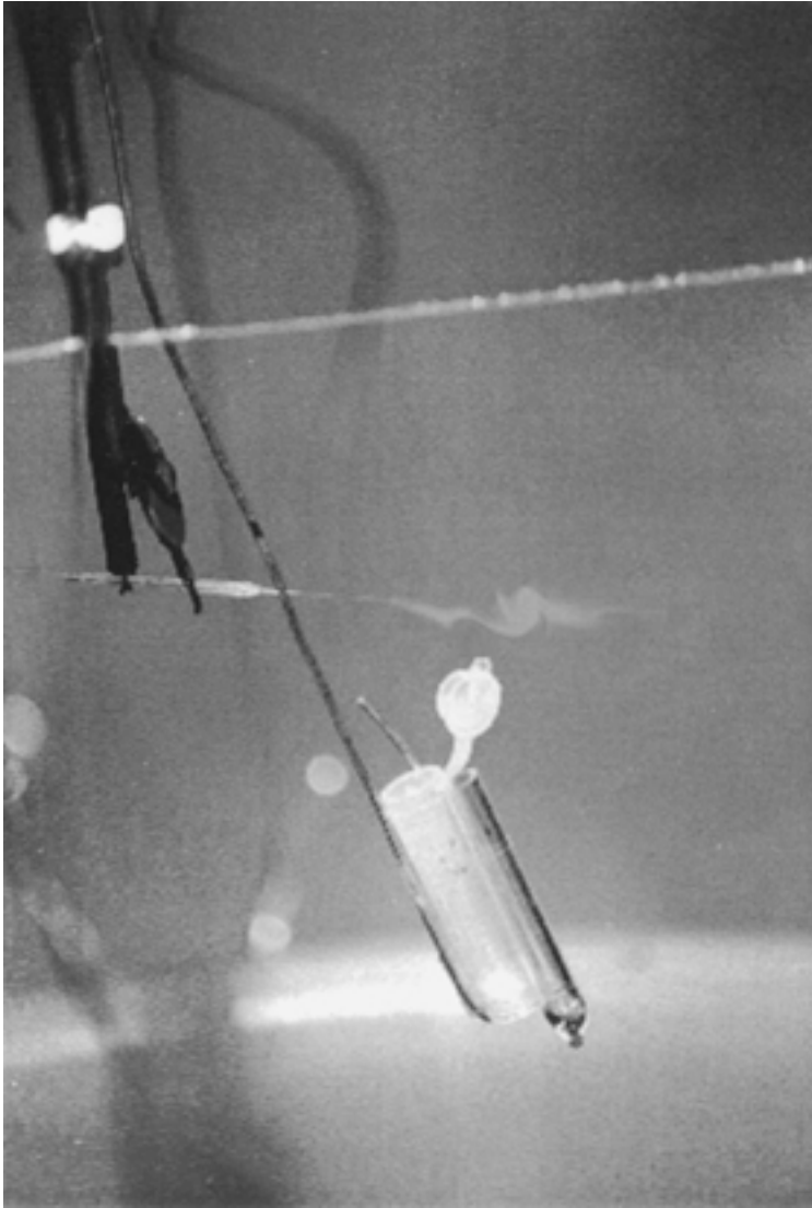
FIG. 3. Photograph of the active sprayer installed in a rotating trap for investigating the effect of Scotch pine monoterpenes on the attraction of P. bidentatus to its aggregation pheromone components in the field. (A) tubing, (B) capillary tube, (C) piezo disk, (D) aerosol of solvent containing semiochemicals, (E) standard polyethylene and glass dispenser tubes (F), and edge of plastic funnel in background.
